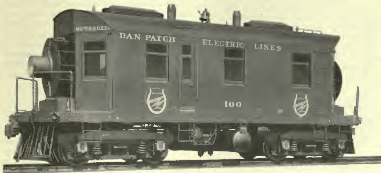
FIG. 440. GASOLINE-ELECTRIC LOCOMOTIVE OF THE "DAN PATCH" LINE
